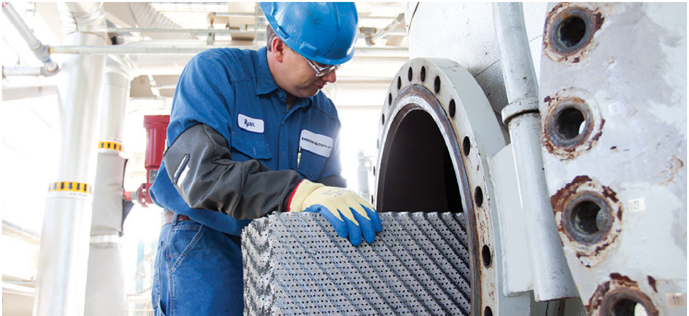
FLEXIPAC® structured packing with a perforated and textured surface.
