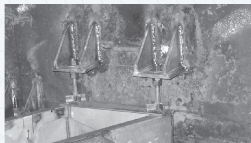
SPECIAL UPLIFT PROTECTION DESIGN FOR A PARTING BOX OF A LIQUID DISTRIBUTOR
