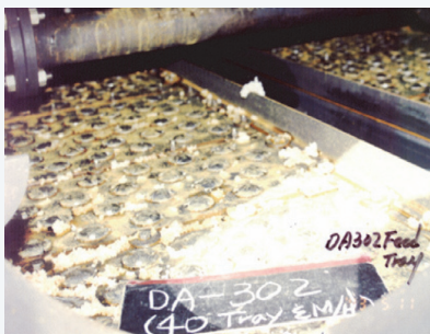
CONVENTIONAL TRAYS SHOW SEVERE FOULING
