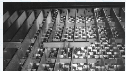
HOLD DOWN GRID WITH THROUGH ROD FOR A STRUCTURED PACKING OR GRID BED
