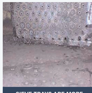
SIEVE TRAYS ARE MORE THAN 90% PLUGGED AFTER 5 MONTHS
