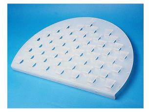
The key to the PROVALVE tray is its proprietary fixed-valve design with a uniquely tapered cover. The cover provides a forward-lateral push to the liquid across the tray, which improves liquid distribution and protects the tray deck from fouling.
