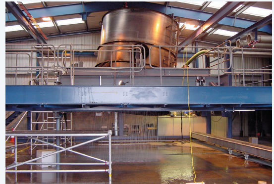
TESTING OF MODEL 961 ENCLOSED CHANNEL DISTRIBUTOR IN THE KOCH-GLITSCH TEST FACILITY SIMULATING WAVE MOTION
