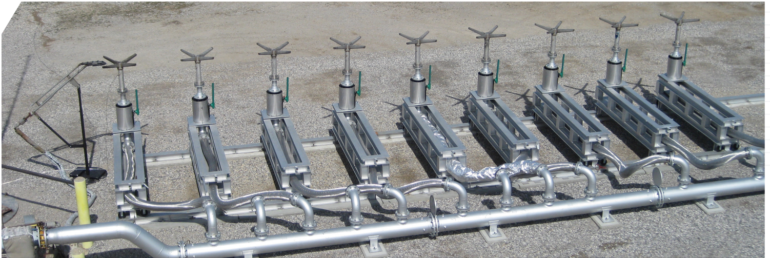
Our unique multi-burner test facility can achieve multiple burner configurations via a rail-system that enables multi-dimensional movement of full-scale burners.
