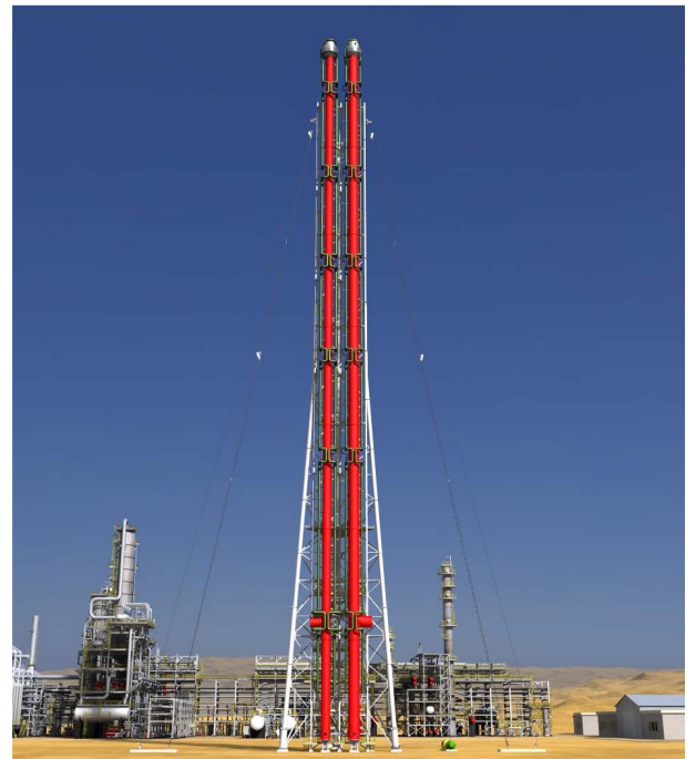
Demountable flares allow flare tip replacement with adjacent flares in service.
