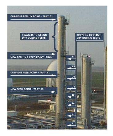
The empirical O'Connell correlation can be used to predict overall column efficiencies (Eoc) for ULTRA-FRAC trays. With this **Test and Demonstration** unit, we can confidently predict ULTRA-FRAC efficiencies.
