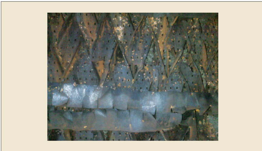
Figure 4 Structured packing after a few months of operations
