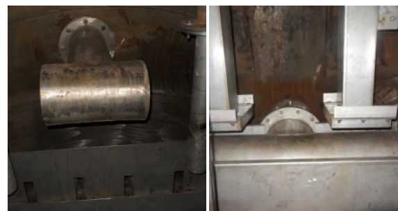
Figure 5. The feed section before (left) and after (right) modification.
