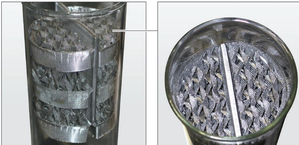
*Miniplant dividing wall column with Montz-Pak A3-1000*
