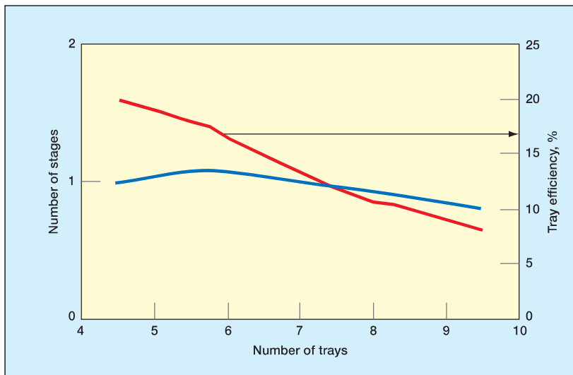
Figure 7 An observed set of tray separation stages for different tray counts in operating vacuum units. The tray count appears to be insensitive to the actual number of stages (approximately one), represented in a reduced tray efficiency
