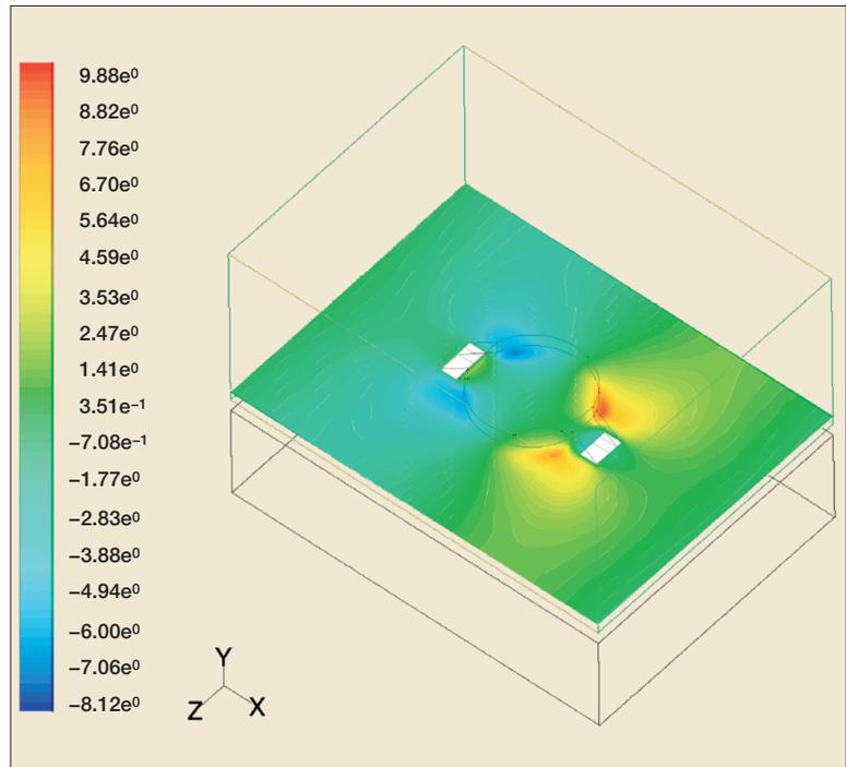
**Figure 6** Computational fluid dynamics (CFD) study for single VG-0 valve
