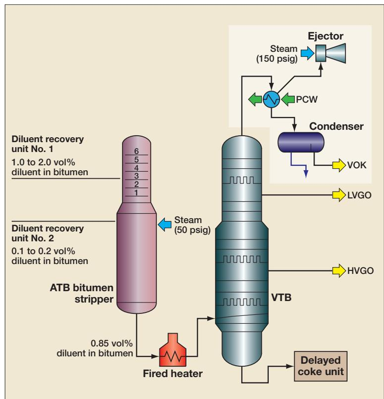
Figure 1 Simplified process flow diagram (the pink tower is the steam stripping tower)
