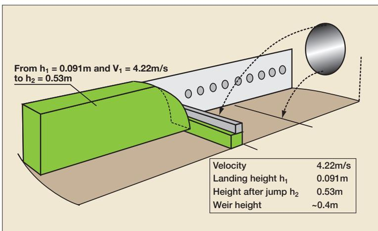
Figure 3 Hydraulic jump calculations for existing liquid inlet
