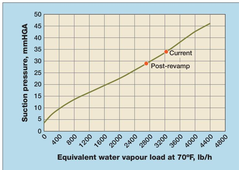
Figure 8 Vacuum overhead pressure comparison
