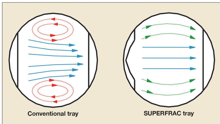
**Figure 7** Liquid flow distribution comparison between conventional trays and multi-chordal Superfrac tray
