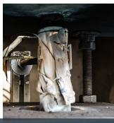
Battery and test plaque before and after thermal runaway.
