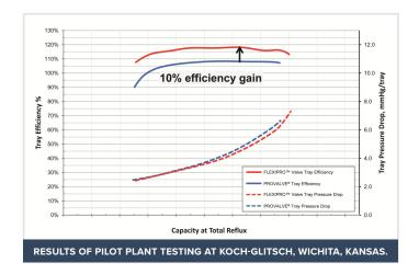
The increased jet flood capacity and reduced weeping has resulted in an operating range that allows the FLEXIPRO® valve tray to be used where moving valves traditionally are applied, but without any of the reliability shortcomings of moving valves.
